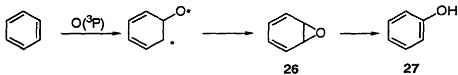
Figure 13. Triplet oxygen reaction with benzene.
